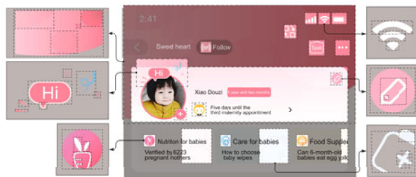
Fig. 1 Examples of fragmented layers in user interface (UI) components (the dashed rectangles represent the fragmented layers). These fragmented layers form UI components with semantic information
