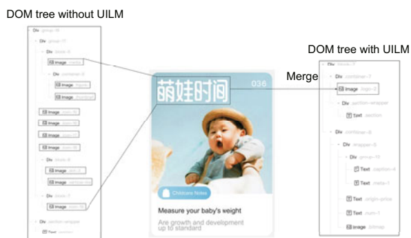
Fig. 11 An example of a generated DOM tree with and without UILM. In the DOM tree without UILM, the dashed boxes represent redundant containers. In the DOM tree with UILM, the single image container represents the “text-like” UI component (DOM: document object model; UI: user interface; UILM: UI layers merger)
